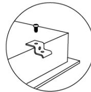
5. The brackets position can be adjusted to suit different thickness of work surfaces:
