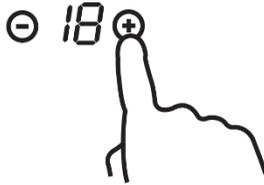
3. When the time is set, it will begin to count down immediately. The display will show the remaining time and the timer indicator will flash for 5 seconds.
